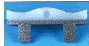
■ Cross section shows how the polyethylene spacer is moulded into the tantalum base plate.
